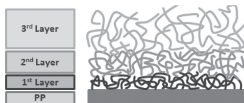
Figure 2. Schematically representation of water-swollen POx multilayers.
